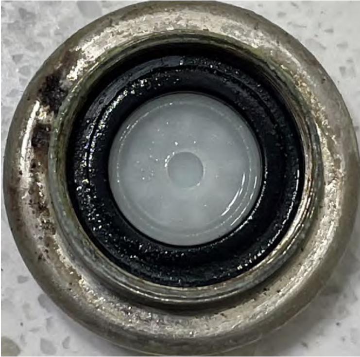
Figure 3. Interior view of master bathroom sink aerator. Upon visual inspection, no debris was observed.
