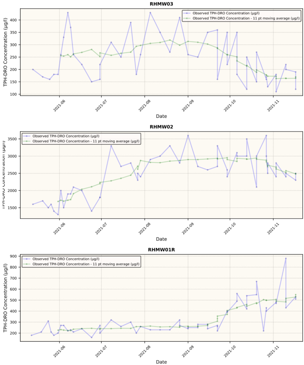
Chart 5-4: TPH-d Concentrations at RHMW03, RHMW02 and RHMW01R Following May 2021 Release with 11-Point Moving Average Used for PEST Simulations as Target Data
