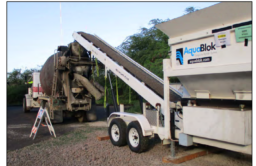
AC material manufacturing on-site
