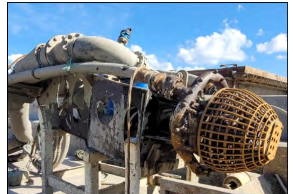
Intake screen to capture MEC during offloading
